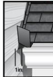
Figure 9 Gutter to Siding
